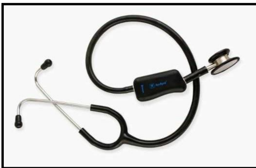
AyuSynk Module attached with conventional stethoscope
